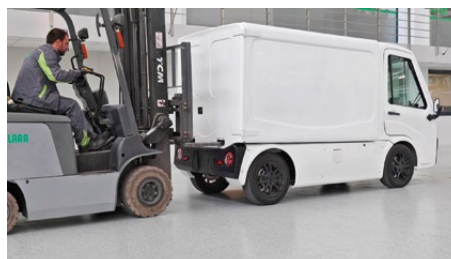
1 Easily changing cargo box with a forklift
